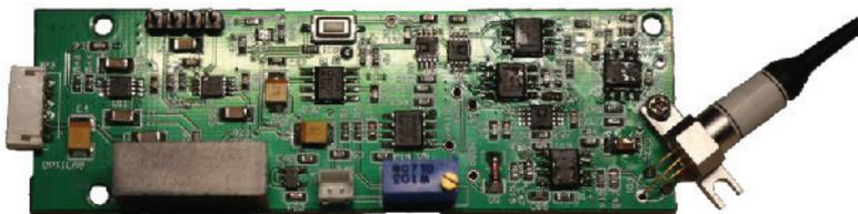
The Optilab M-CB is a compact bias control board designed for M-APE-I-1550-20 modulator
